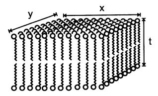
The thickness, t, is restricted to  $t = 2\ell max$ . Thus, v = 2(1.26Nc + 0.84)(x)(y). Calculation of m gives
