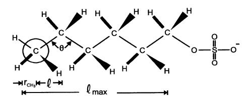
The projection of the C-C bond length,  $\ell$ , along the chain axis is  $\ell=1.54 \sin(109^{\circ}54'/2)=1.26$  Å. Thus  $\ell_{\text{max}}=(\text{Nc}-1)(1.26)+r_{\text{CH}_3}$ , where  $r_{\text{CH}_3}=2.1$  Å, the radius of the terminal -CH<sub>3</sub> group. Finally,
